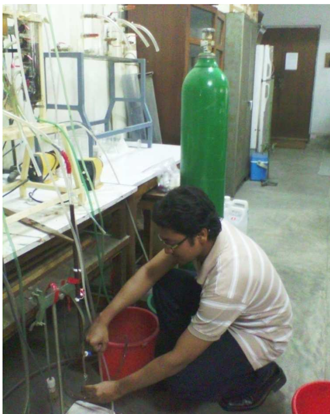
Figure B9: Collecting effluent sample from glass burette during laboratory column experiment to calculate Mn concentration
