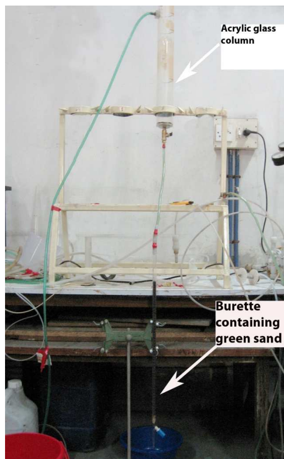
Figure 3.1: Experimental set up for Mn removal mechanism study
