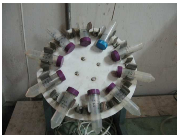
Figure 3.3: Tilted rotator used for batch experiment to determine Mn uptake capacity of green sand media.
