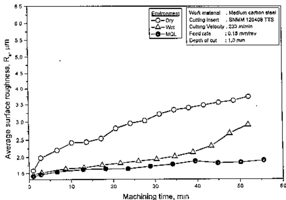
**Fig.4.8** Variation in surface roughness with progress of turning steel by coated carbide insert under dry, wet and MQL conditions.
