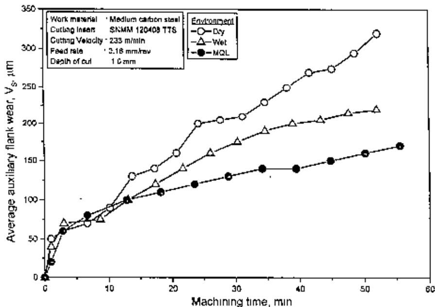
**Fig.4.2** Growth of average auxiliary flank wear with machining time under dry, wet and MQL conditions
