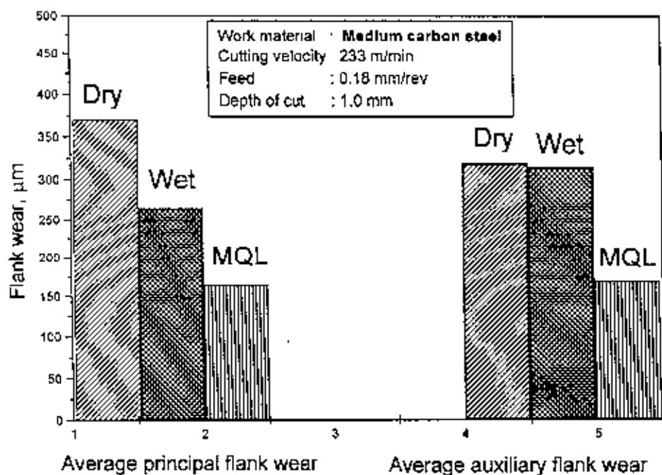
Fig. 4.4 Flank wear developed in insert after machining steel for 52 minutes under **dry**, **wet** and **MQL** conditions.
