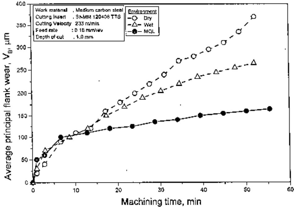
Fig.4.1 Growth of average principal flank wear with machining time under dry, wet and MQL conditions
