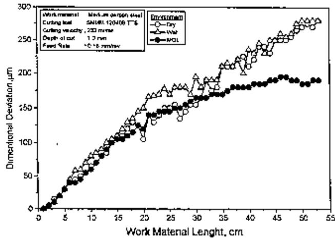
Fig.4.9 Variation in dimensional deviation with progress of turning steel by coated carbide insert under **dry**, **wet** and **MQL** conditions.
