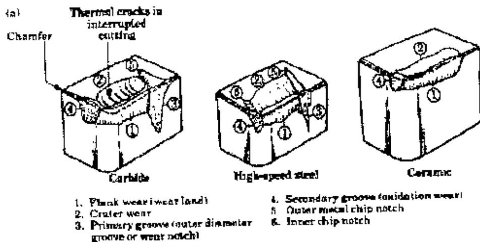
Fig.2.2 Tool wear mechanisms [Kalpakjian 1997]
