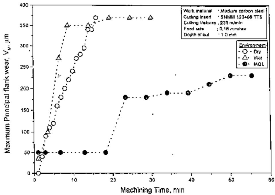
**Fig.4.3** Growth of maximum flank wear,  $V_M$  with machining time under dry, wet and MQL conditions
