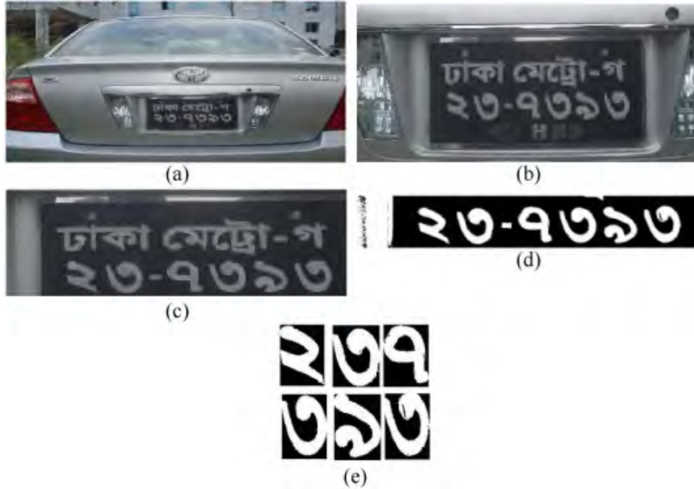
Fig. 3.6: (a)Initial image, (b) The result of applying empirical crop, (c) Image obtained after brute force scanning and cropping, (d) The lower half of the registration plate, and (e) Individual characters being extracted from the registration plate.
