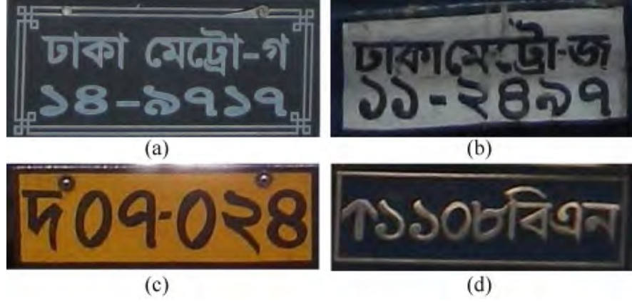
Fig. 1.4: Different types of Bangla license plate: (a) Private, (b) Public, (c) Government, and (d) Military.
