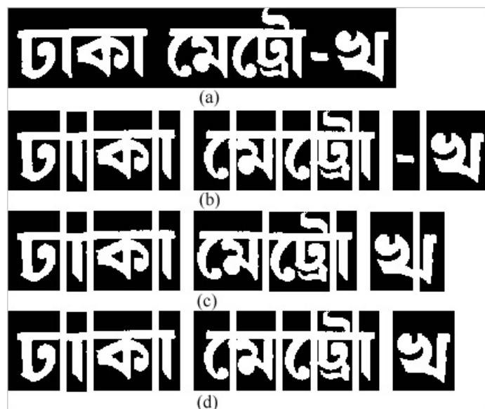
Fig. 5.2: Character segmentation: (a) Original license plate, (b) Manual segmentation, (c) Segmentation with constant threshold [4], and (d) Segmentation with adaptive threshold (Algorithm SAT).
