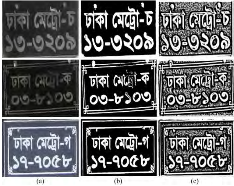
Fig. 2.3: (a) Original input images, (b) Binarization using Otsu's algorithm, and (c) Binarization using Sauvola Algorithm.
