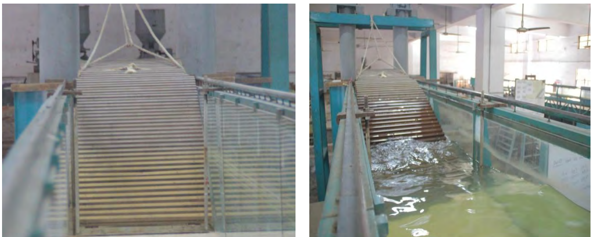
Figure 3.5: Wave absorber to damp the transmitted wave
