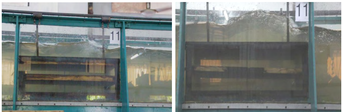
Figure 3.8 (d): Wave breaking near the onshore end of the breakwater
