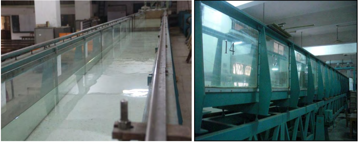
Figure 3.1: Laboratory flume (21.3 m long, 0.76 m wide and 0.74 m deep)
