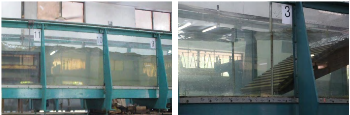
Figure 3.8 (f): Transmitted wave after passing the breakwater
