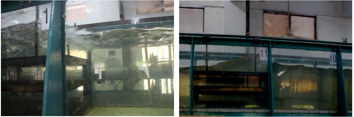
Figure 3.8 (e): Wave breaking just behind the breakwater
