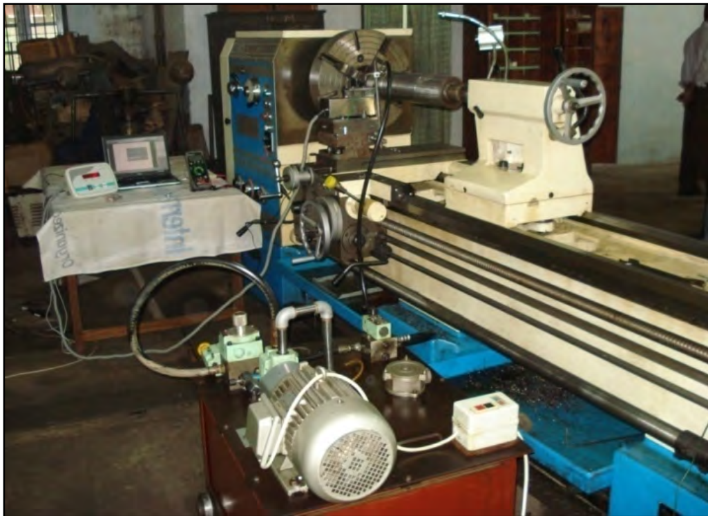
Fig.2.3 Photographic view of the experimental set-up for turning hardened steel with high pressure coolant (HPC) jet
