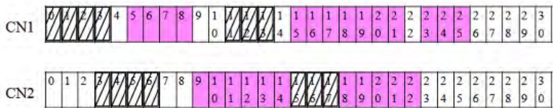
Figure 3.13: Status of the CN s after T_4 and T_5 are mapped in the Second Iteration
