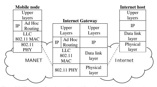
Figure 2.7: The protocol stacks used by mobile nodes, gateways and Internet hosts.
