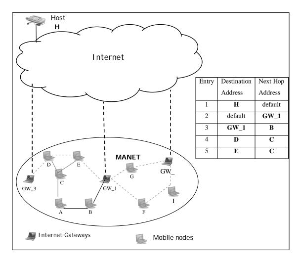
Figure 4.2: Routing table of a mobile node in our scheme
