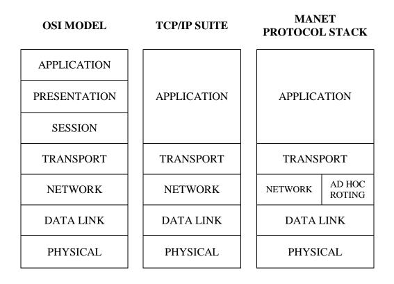
Figure 2.2: The OSI model, TCP/IP suite and MANET protocol stack.
