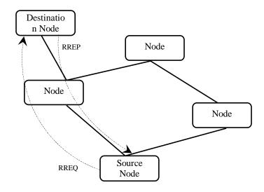
Figure 2.4: Ad Hoc On-Demand Distance Vector Routing Protocol
