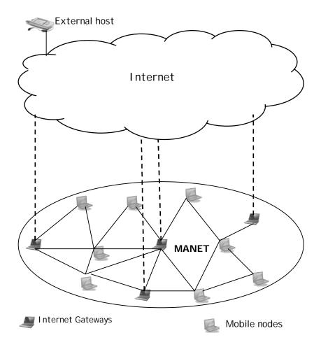
Figure 4.1: Network architecture to connect MANET to the Internet
