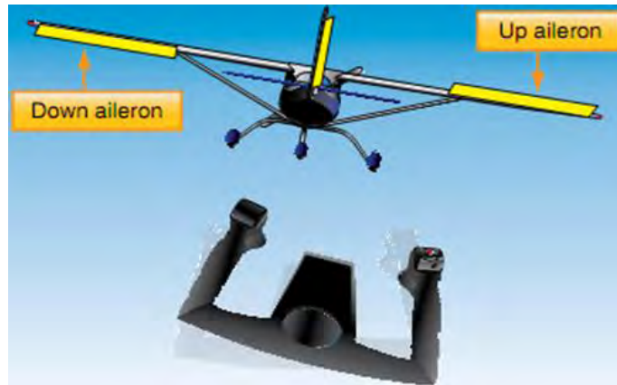
Figure 2.3: Aileron working principle (looking from aft) [39]
