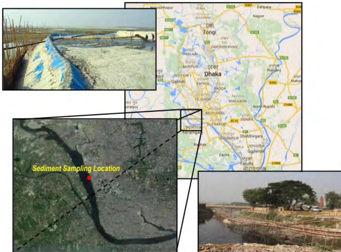
Figure 3.1 Sediment sampling location in the Buriganga River. Inset pictures show pipelines that are used to convey riverbed sediments for land filling purpose.
