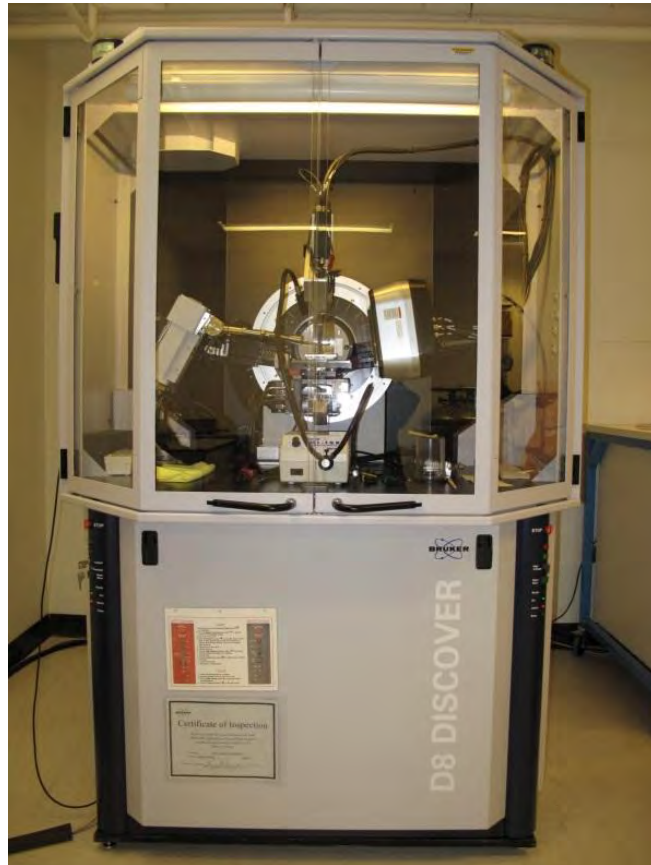
Figure 3.5 Bruker D8 X-ray Diffractometer.
