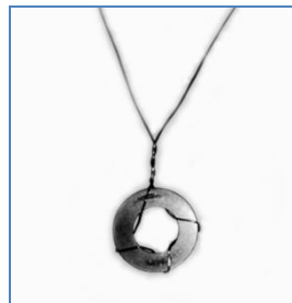
Figure 3.10 Toroid shaped sample for permeability measurement.
