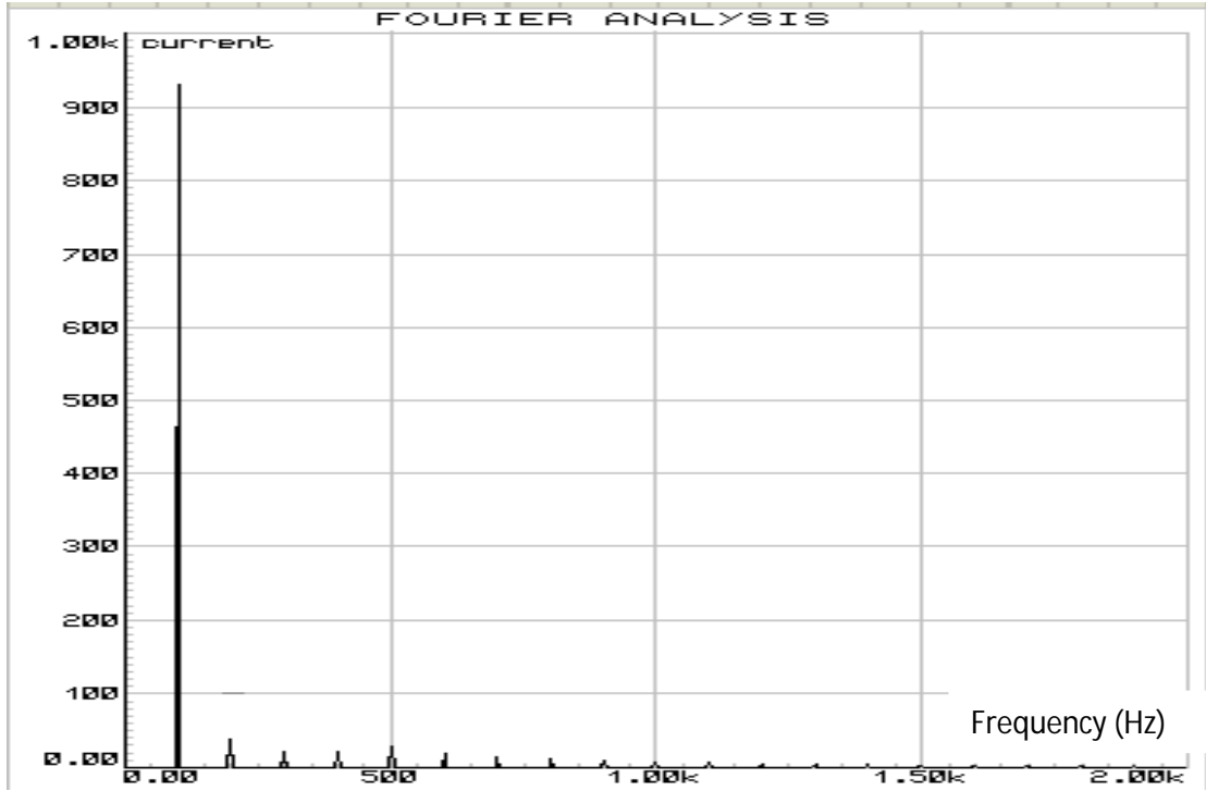
Fig 3.28 FFT component of input current for 800Ω load resistance and 325V (peak) input voltage
