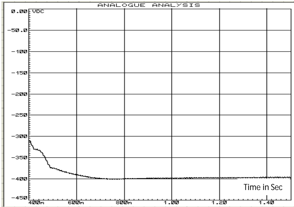
Fig 3.52 Output voltage for 200Ω load resistance and 367V (peak) input voltage
