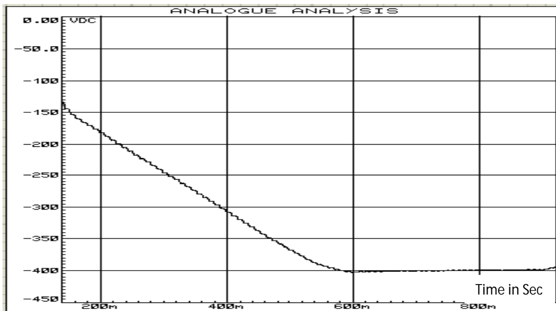
Fig 3.62 Output voltage for 400Ω load resistance and 55Hz input frequency
