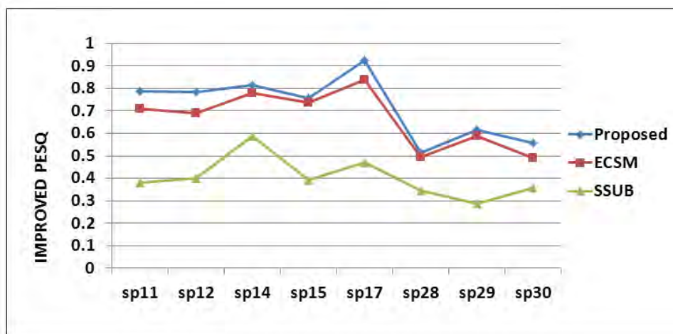
Fig. 4.19: PESQ improvement comparing proposed method, ECSM method and SSUB method in case of white noise corrupted signal at SNR of 10 dB for a subset consists of eight speech sentences of NOIZEOUS database.
