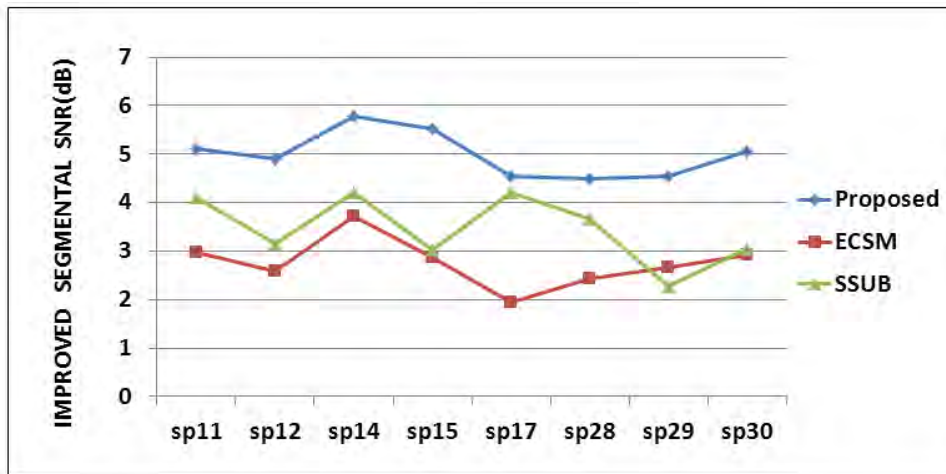
Fig. 4.15: Segmental SNR improvement comparing proposed method, ECSM method and SSUB method in case of white noise corrupted signal at SNR of 5dB for a subset consists of eight speech sentences of NOIZEOUS database.
