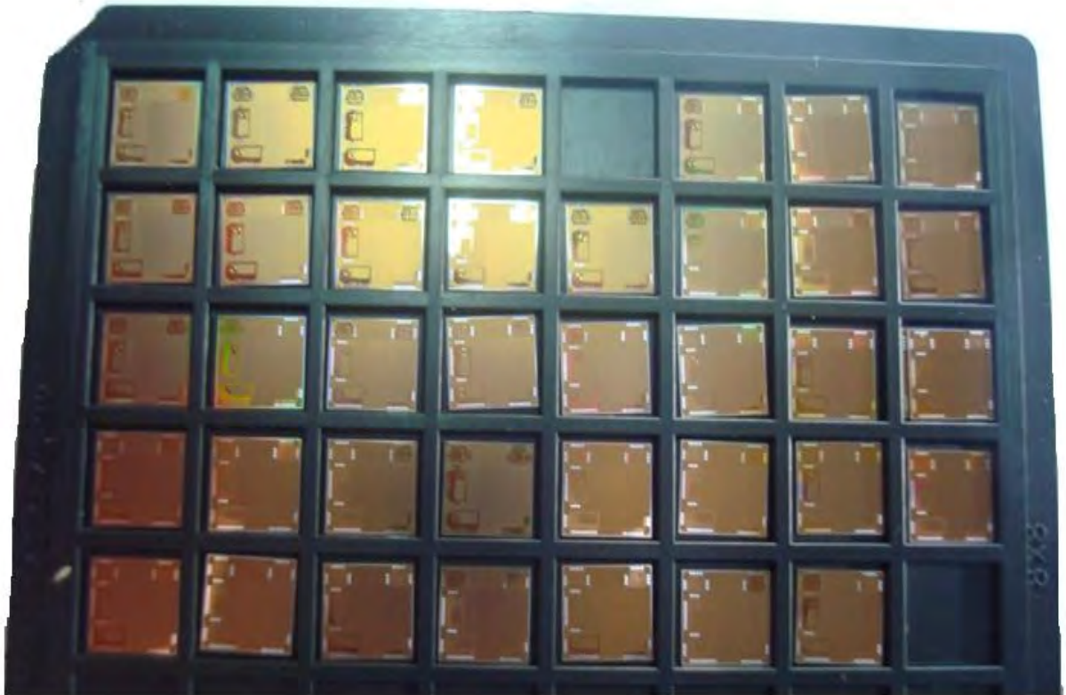
Figure A.1: Photograph of the lot of 40 chips of 21 GHz source degenerated LNA
