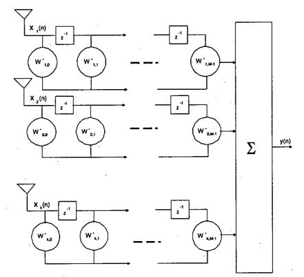
Figure 2.6: Wideband beamforming
