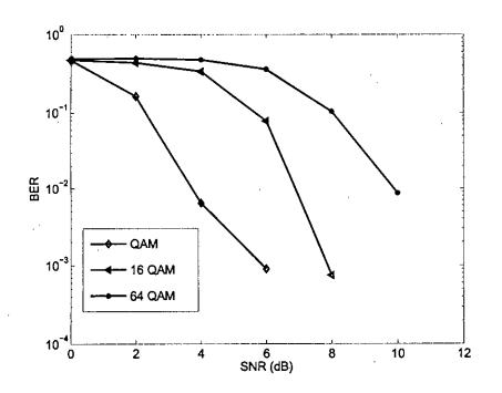
Figure 5.4: BER vs. SNR for different quadrature amplitude modulation for coded OFDM with multiple antennas
