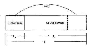
Figure 3.9: Insertion of guard time
