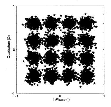
Figure 3.7: Example IQ demodulation constellation. 16-QAM
