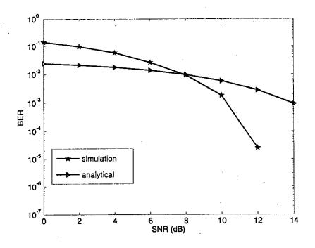
Figure 5.10: BER vs. SNR for OFDM with analytical value and simulation value
