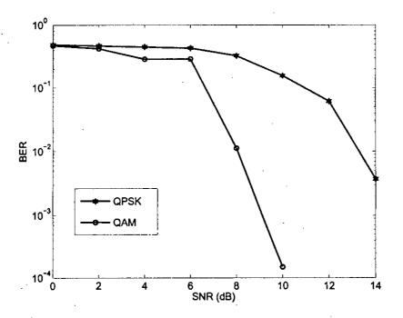
Figure 5.5: BER vs. SNR for different modulation for coded OFDM with multiple antennas
