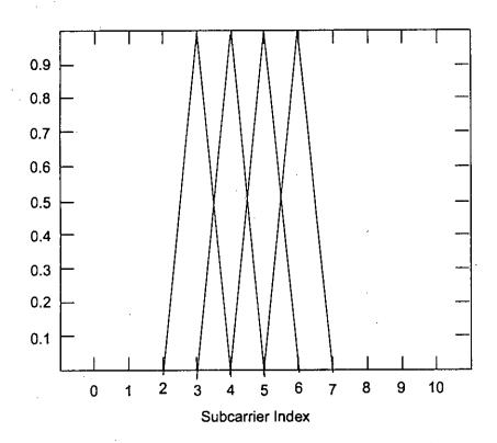
Figure 3.2: Spectra of four orthogonal subcarriers
