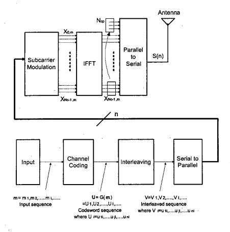
Figure 4.3: Discrete time baseband equivalent model of an OFDM transmitter
