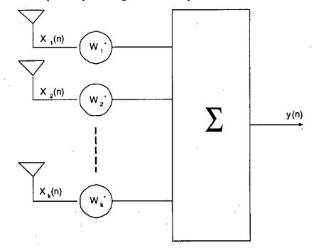
Figure 2.5: Narrowband beamforming
