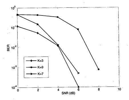
Figure 5.8: BER vs. SNR for OFDM for different constraint length for coded OFDM with multiple antennas
