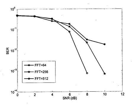
Figure 5.7: BER vs. SNR for different FFT length for coded OFDM with multiple antennas
