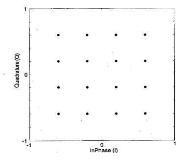
Figure 3.6: Example IQ modulation constellation. 16-QAM
