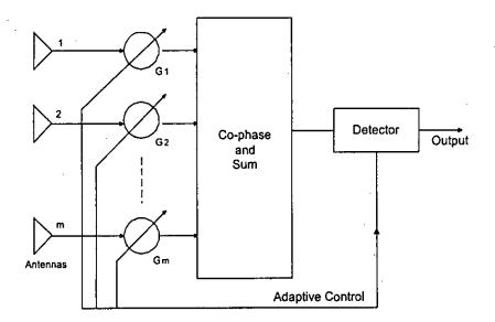
Figure 2.4: Block diagram of a maximal ratio combiner
