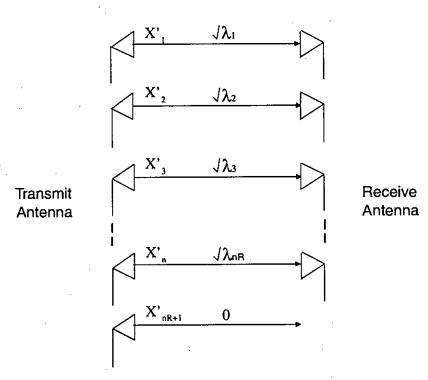
Figure 4.10: Equivalent uncoupled MIMO channel for nT > nR
