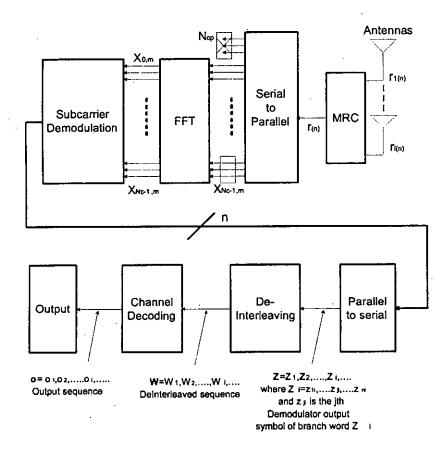
Figure 4.4: Discrete time baseband equivalent model of an OFDM receiver
