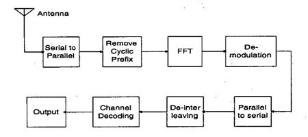
Figure 3.10: Block diagram of an OFDM receiver with single antenna
