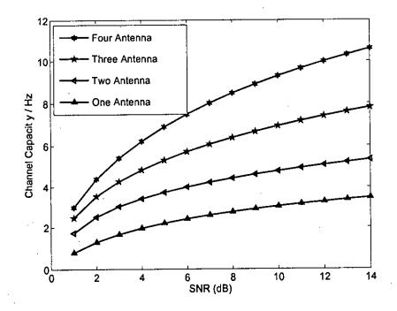
Figure 5.13: channel capacity enhancement by increasing number of antennas
