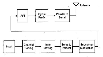
Figure 3.3: Block diagram of an OFDM transmitter
