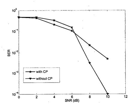
Figure 5.6: BER vs. SNR for different cyclic prefix length for coded OFDM with multiple antennas
