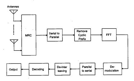
Figure 4.2: Block diagram of the proposed OFDM receiver with multiple antennas
