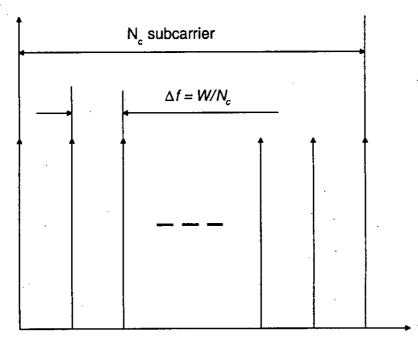
Figure 3.1: Subdivision of the bandwidth into Nc subbands
