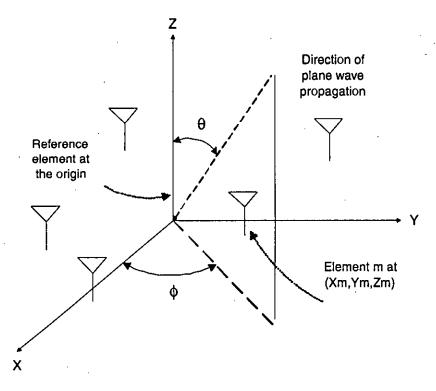
Figure 2.2: Co-ordinates of an antenna array
