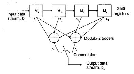
Figure 3.4: Convolutional encoder
