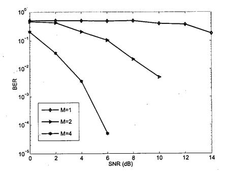
Figure 5.2: BER vs. SNR for coded OFDM with different number of antennas
