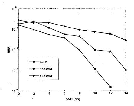
Figure 5.3: BER vs. SNR for different quadrature amplitude modulation for uncoded OFDM with multiple antennas
