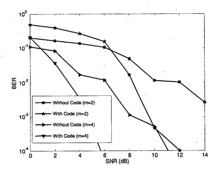
Figure 5.9: BER vs. SNR for OFDM with and without coding and interleaving for multiple antennas
