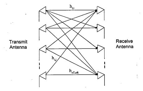
Figure 4.9: Multiple input multiple output channel of wireless network
