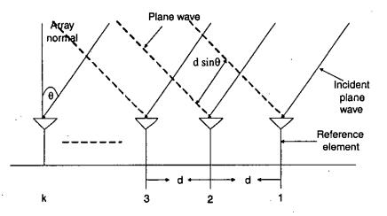
Figure 2.1: A uniformly spaced linear antenna array written as [31]
