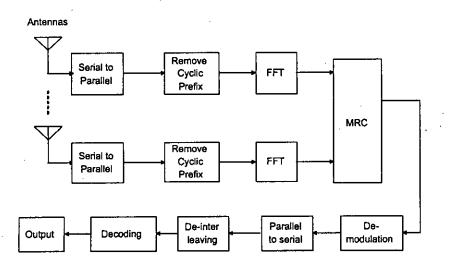
Figure 4.1: Block diagram of a conventional OFDM receiver with multiple antennas
