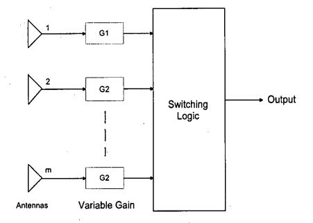
Figure 2.3: Block diagram of a selection combiner
