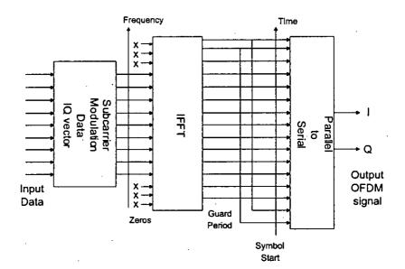
Figure 3.8: OFDM generation at IFFT stage
