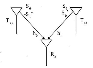
Figure 4.11: Single input multiple output for two antenna case
