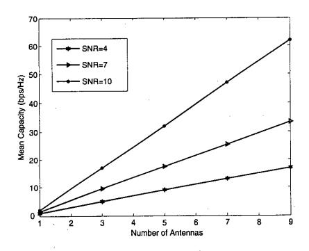
Figure 5.12: Mean channel capacity enhancement by increasing number of antennas
