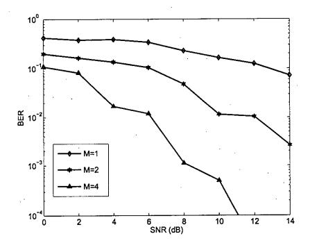
Figure 5.1: BER vs. SNR for OFDM without coding and interleaving for different number of antennas
