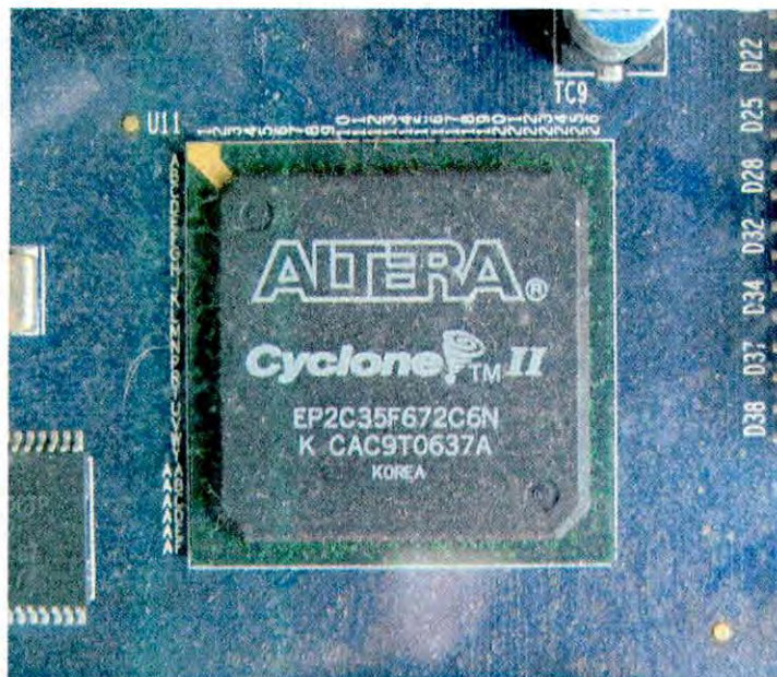
Figure 4.6 Cyclone II FPGA chip in DE2 board
