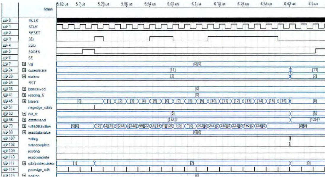
Figure 5.5 State 4. Setting sampling rate 1kHz.
