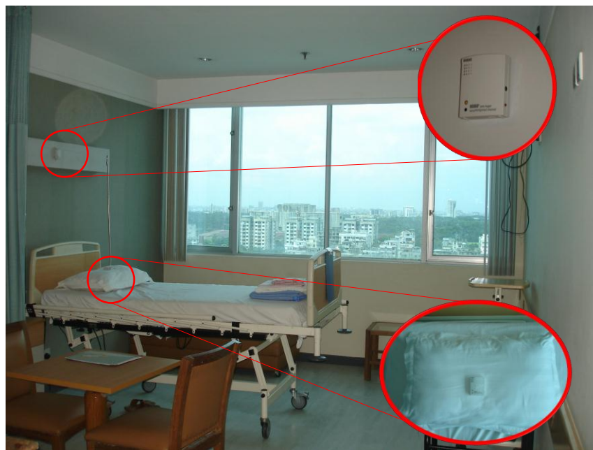
Figure 3.6: Placement of additional data loggers on a vacant bed.
