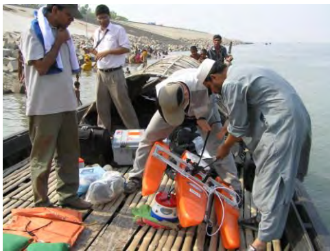
(a) ADCP is being connected with plastic boat (b) ADCP is prepared for data collection
