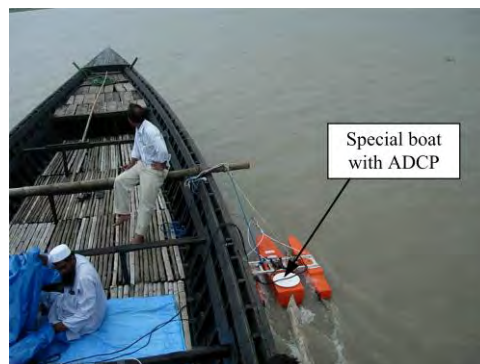
(c) Data is being collected using ADCP
