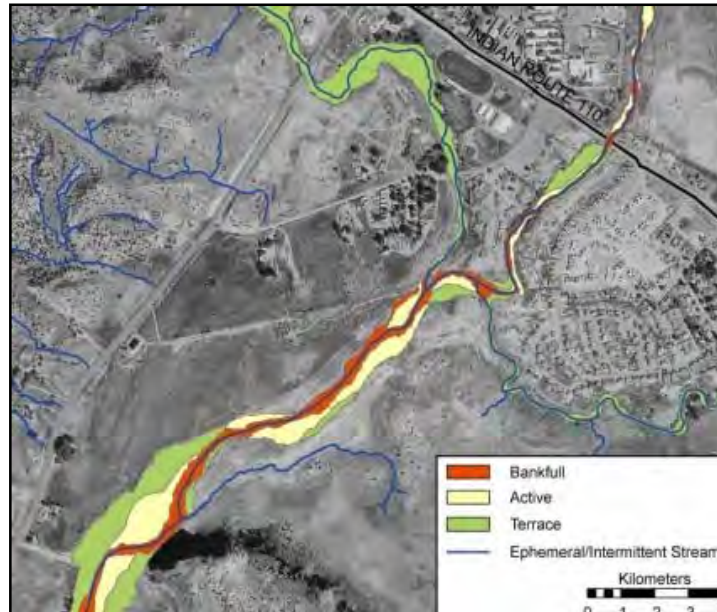
Figure 2.4 Floodplain delineation by HEC-RAS hydrologic model (USACE, 2009)
