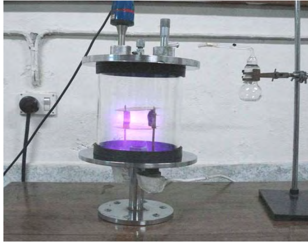
Figure 3.4 Plasma polymerization system in laboratory.
