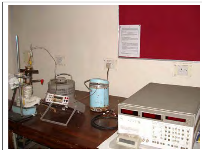
Figure 3.14 Photographs of the ac electrical measurement set-up.
