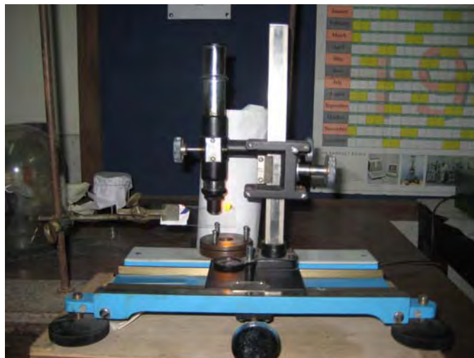
Figure 3.7 Interferometer arrangements in the laboratory
