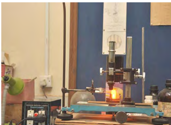
Fig. 4.9 Traveling microscope arrangement for film thickness measurement.
