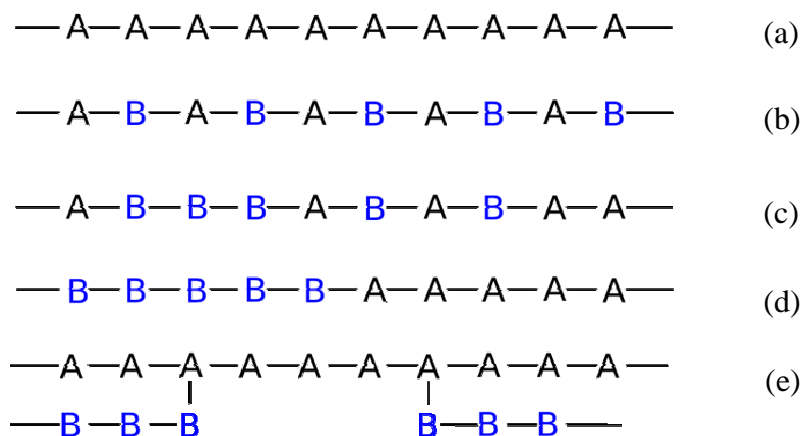
Fig. 2.4 Types of copolymers (a) Homopolymers, (b) Alternating copolymer, (c) Statistical copolymers, (d) Block copolymers and (e) Graft copolymers.
