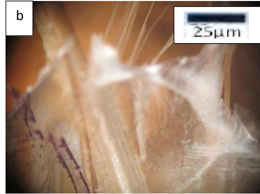
Figure 4.106 Optical micrographs of tensile fracture surface of (a) horizontal and (b) surface for UD+45°+90° raw bamboo fiber containing composite.
