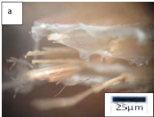
Figure 4.107 Optical micrographs of tensile fracture surface of (a) horizontal and (b) surface for 15% BCS grafted bamboo fiber containing composite.
