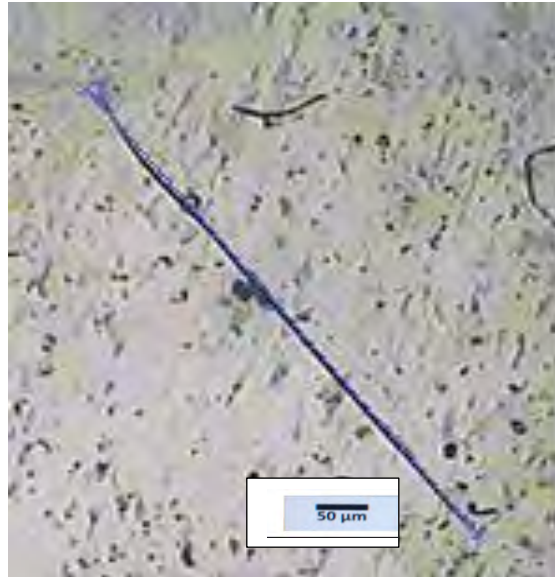
Figure 4.22 Optical image of delignified raw bamboo sample for fiber length determination.
