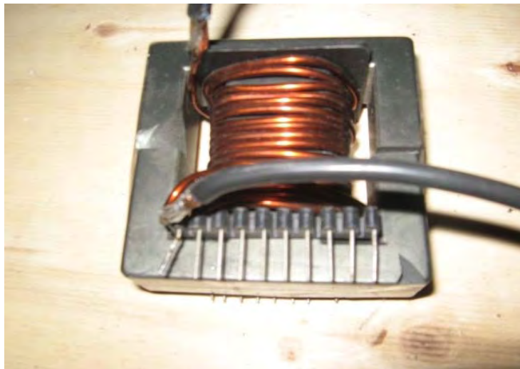
Figure 4.12: Inductor of 1.01mh
