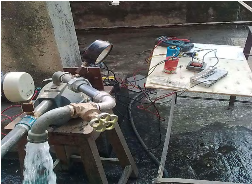
Figure 4.17: Solar Water Pump with BUCK converter
