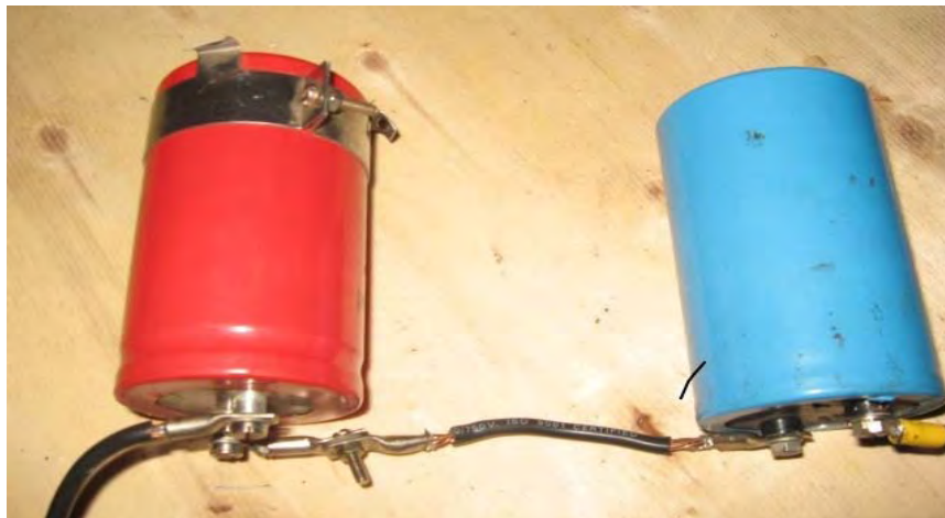
Figure 4.13: One of the Capacitor Banks
