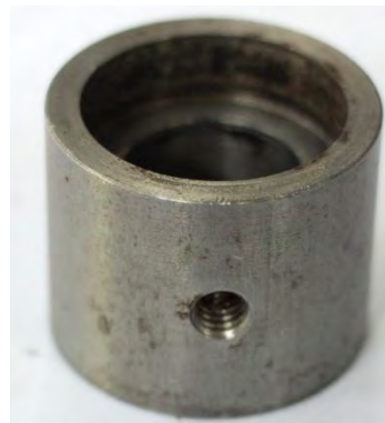
Fig.2.4 Photographic view of liquid nitrogen container for rotary liquid nitrogen applicator
