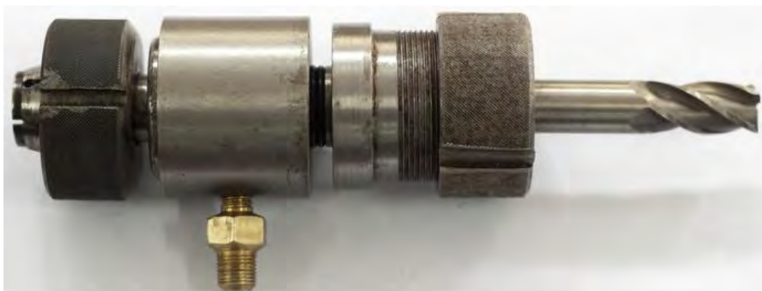
Fig.2.8 Photographic view of rotary liquid nitrogen applicator for injecting liquid nitrogen during milling operation
