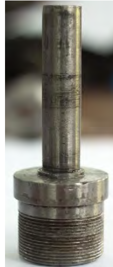
Fig.2.3 Photographic view of adapter for rotary liquid nitrogen applicator
