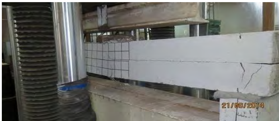
Figure 4.25 Failure Pattern of Specimen-HB53C
