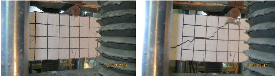
Figure 4.8 Failure Pattern of Specimen-HB37C
