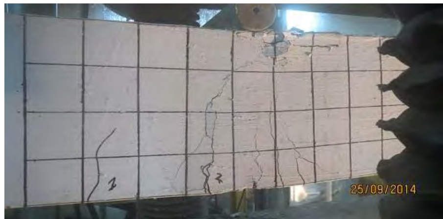
Figure 4.11 Failure Pattern of Specimen-FB4
