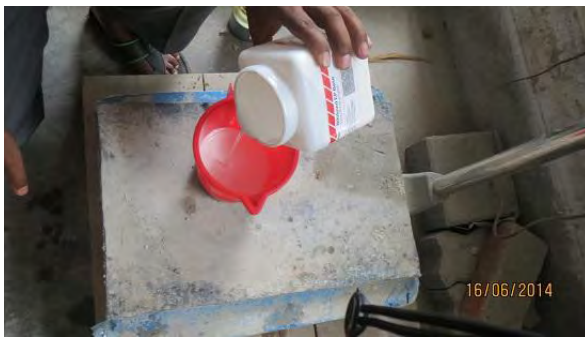
Figure: 3.12 Preparation of 50MPa Epoxy
