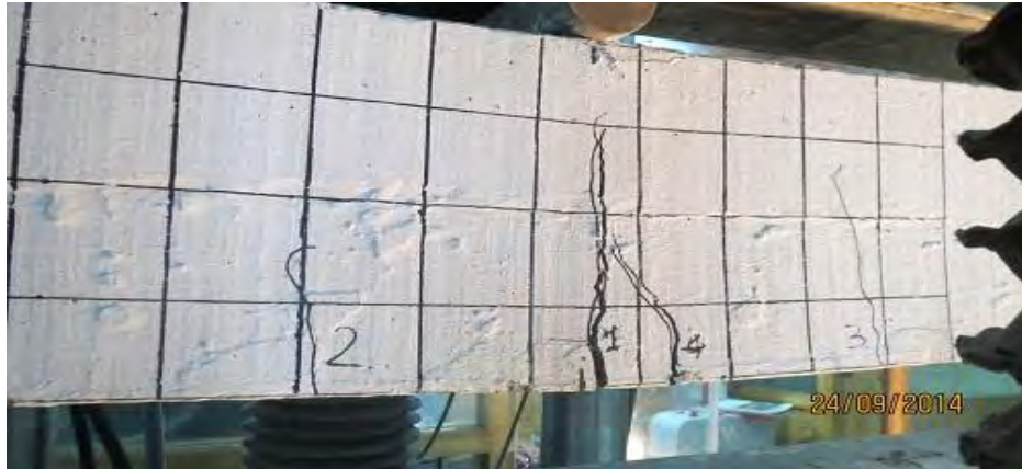
Figure 4.12 Failure Pattern of Specimen-HB41C
