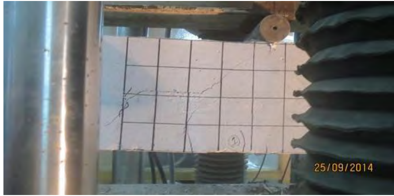
Figure 4.20 Failure Pattern of Specimen-HB47PC
