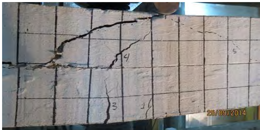
Figure 4.15 Failure Pattern of Specimen-HB43C
