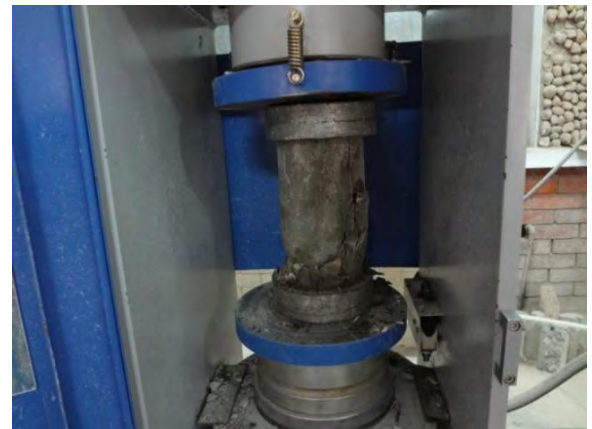
Figure 3.7. Compressive Strength Testing of Cylinders
