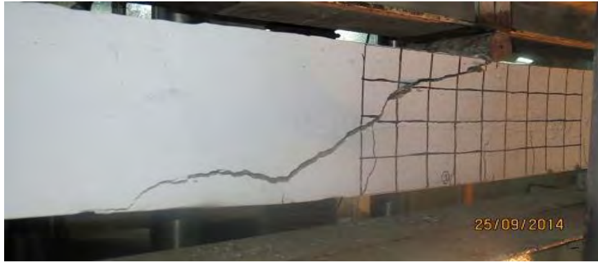
Figure 4.18 Failure Pattern of Specimen-HB47C
