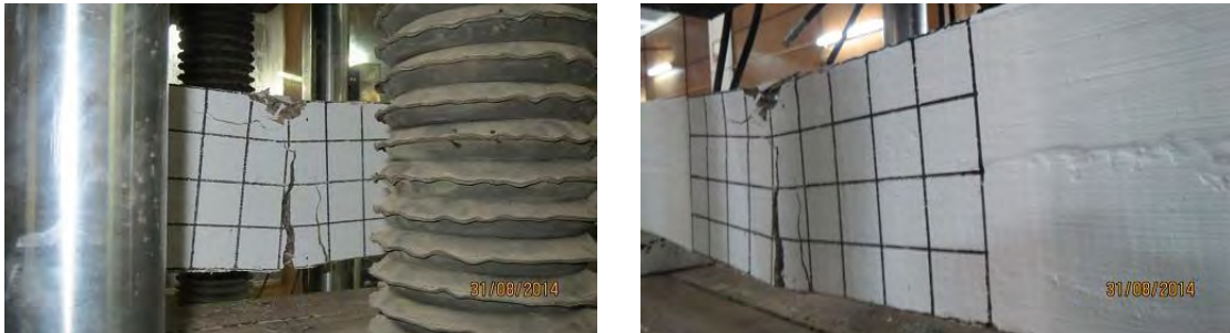
Figure 4.2 Failure Pattern of Specimen-HB31C
