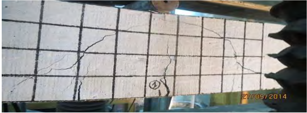
Figure 4.4 Failure Pattern of Specimen-HB31PC
