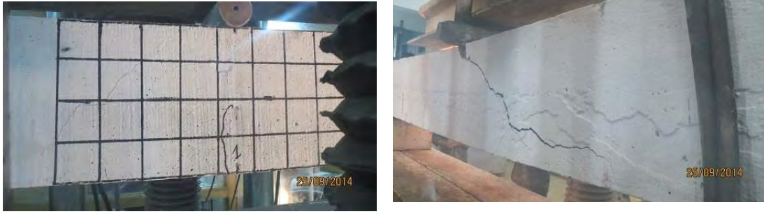
Figure 4.30 Failure Pattern of Specimen-HB57PC
