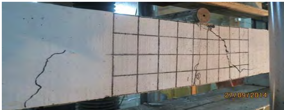
Figure 4.5: Failure Pattern of Specimen-HB33C
