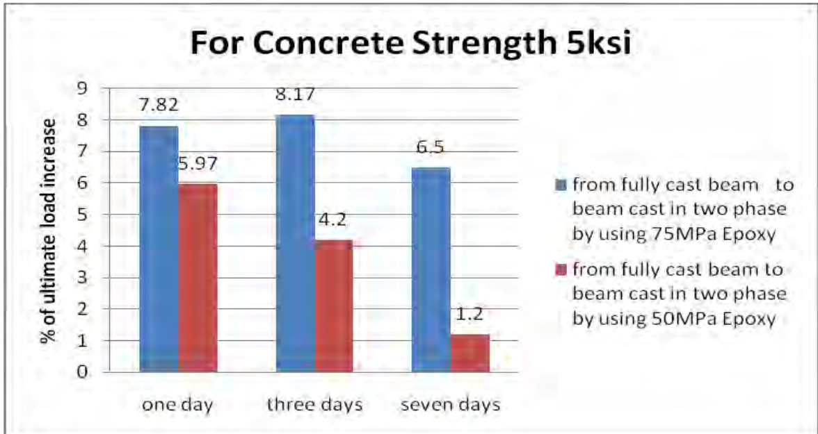
Figure 4.64 Effect of Various Age of Concrete on Ultimate Load for Concrete Strength 5 ksi
