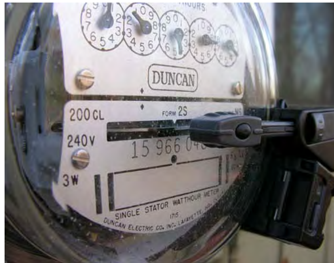
Figure A 2.1: Optical Meter Reader Attached With Electro-Mechanical Energy Meter
