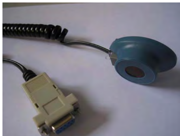
Figure A 2.2: Optical Probe With RS- 232 Port Data Interfacing System
