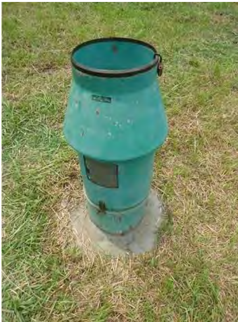
Figure: 2.1 Rain gauges used to measure the amount of rainfall manually
