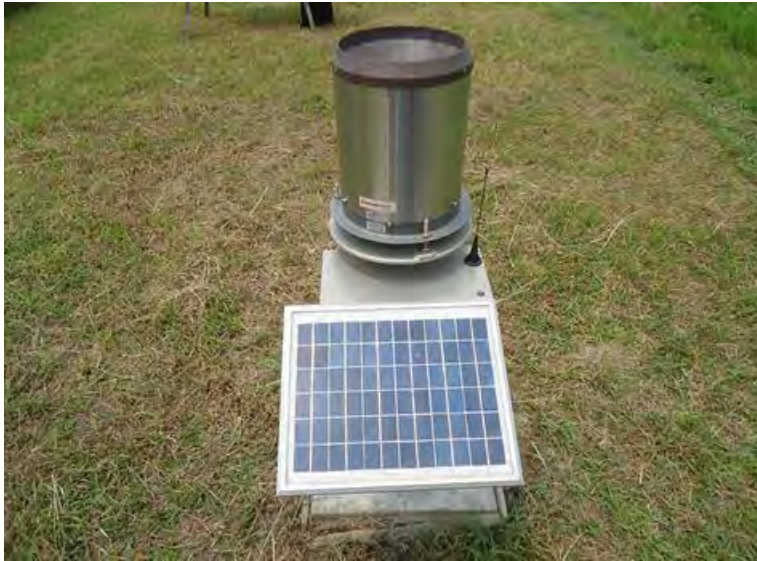
Figure: 2.2 Rain gauges used to measure the amount of rainfall automatically
