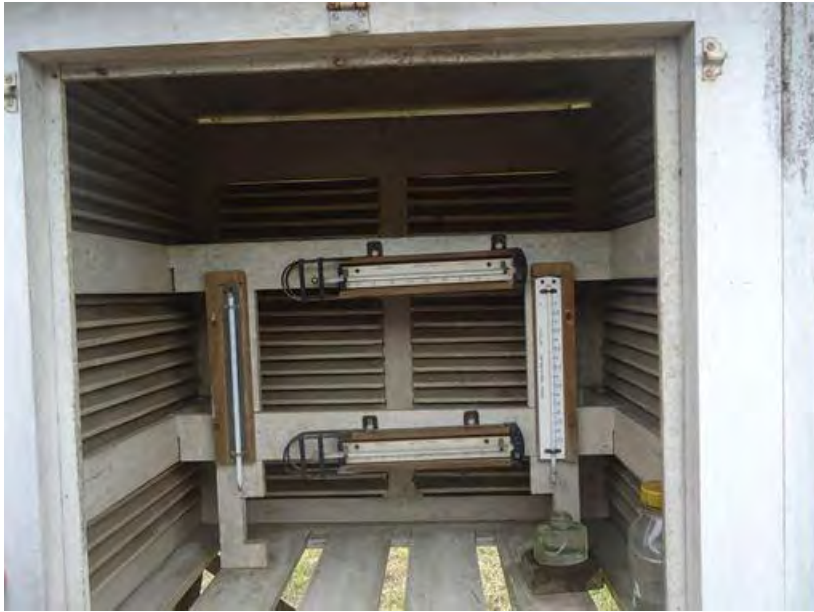
Figure 2.3 Dry, Wet and Maximum, Minimum Thermometer
