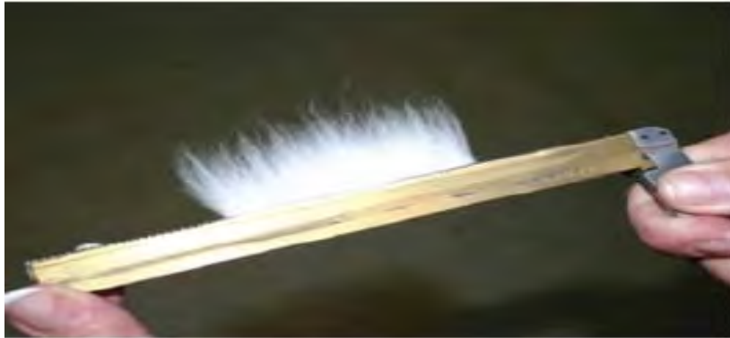
Figure 3.4 Photo of a fibre array comb for the HVI Fibrograph (length) and strength tester. (CSIRO).
