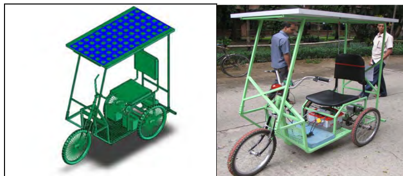
Figure 4.33(b): Finally assembled solar three-wheeler
