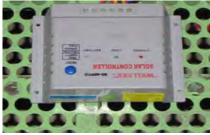
Figure 4.4: MPPT Charge controller
