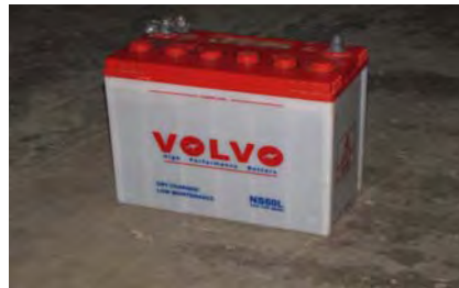
Figure 4.5: Lead acid battery
