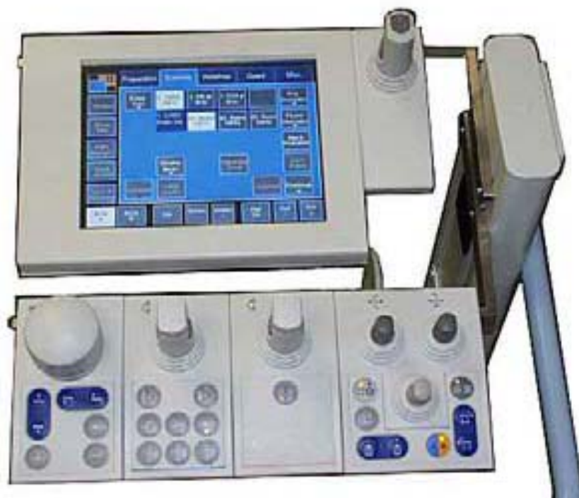
Fig 4.12: Component in the Exam room. ECC, Control module
