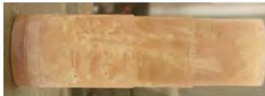
Fig. 2.4 Work material (Kevlar and glass fiber reinforced polyester)
