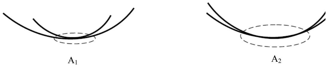
Figure 2.8: Contact area of CwD (right) is smaller than contact area of drill pipe (left) A_1 < A_2 , A = contact area of the pipe with the wellbore( Karimi et al., 2011)
