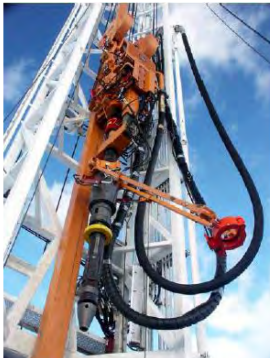
Figure 2.2: Casing Drive System mounted to top drive (Warren et al., 2004)
