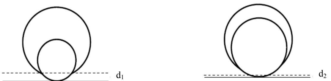
Figure 2.9: Penetration depth onto filter cake, penetration of CwD (right) is less than penetration of drill pipe (left) d_1 > d_2 ; d = penetration depth into the filter cake ( Karimi et al., 2011)
