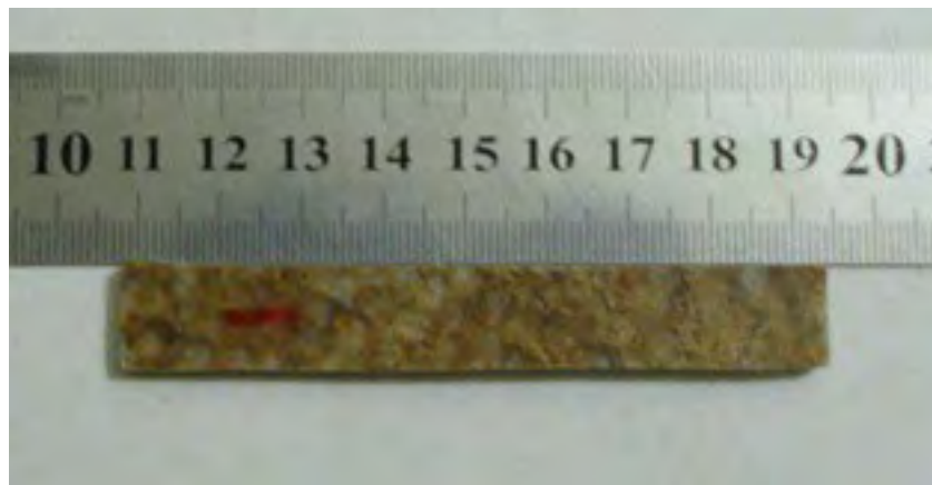
Figure 13 : Photograph of a Flexure test specimen.
