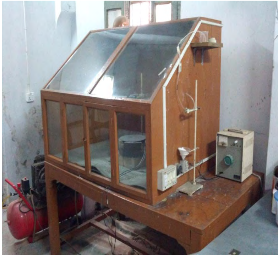
Figure 4.4: Experimental set up of Spray Pyrolysis unit at the Department of Physics, BUET
