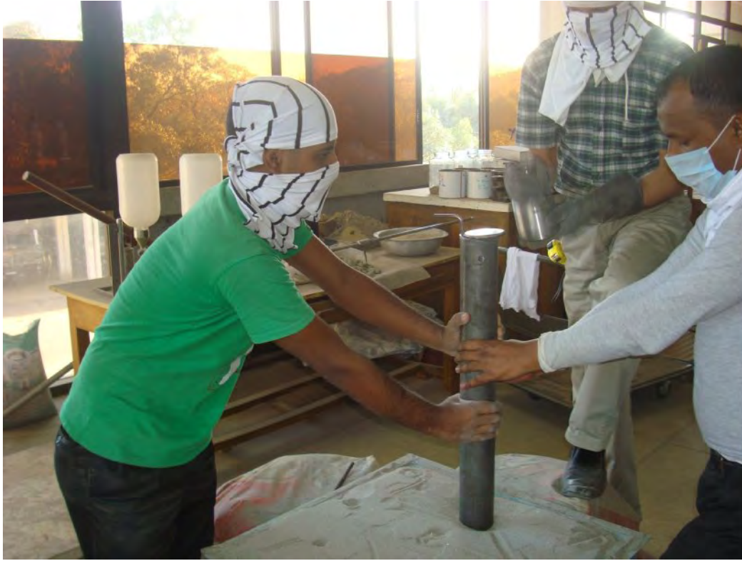
Figure 3.13 (c): Driving of SCP Mandrel
