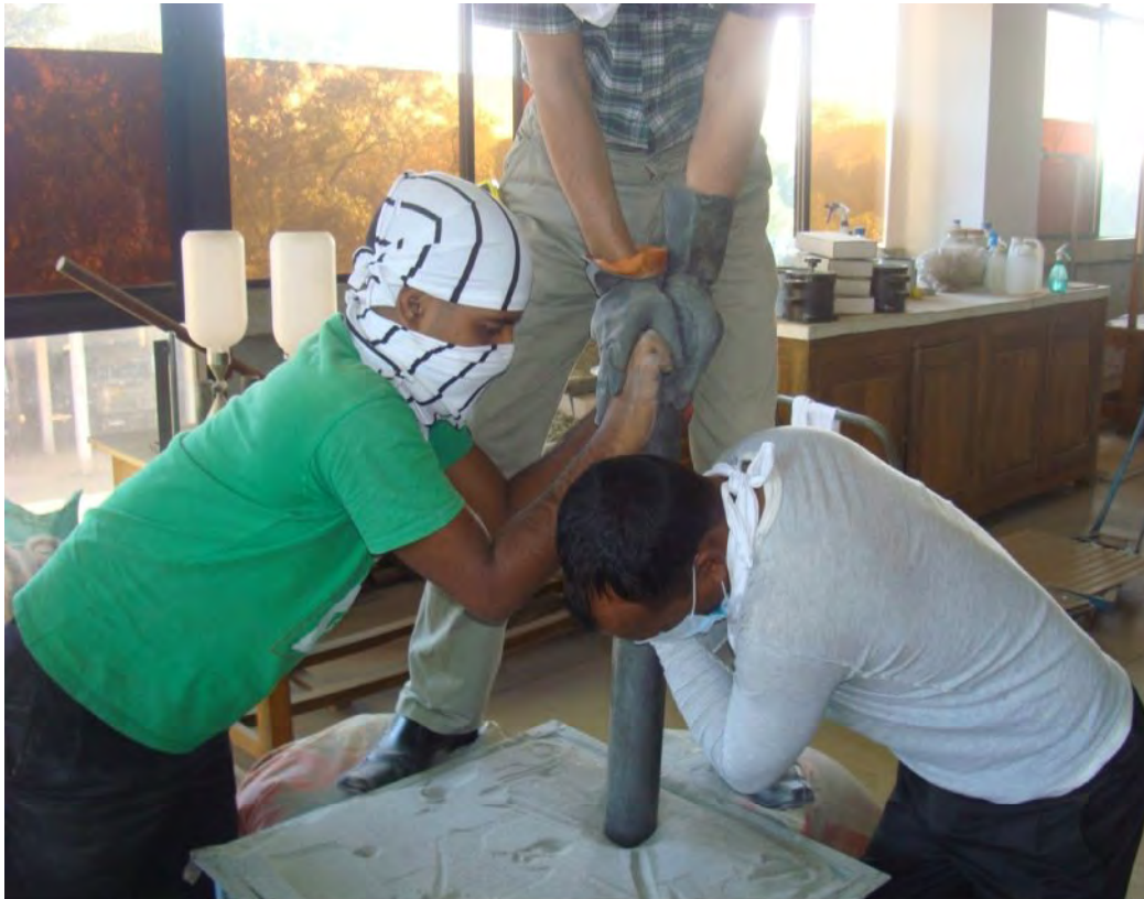
Figure 3.13 (b): Initial Push to the SCP Mandrel
