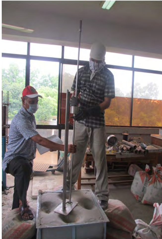
Figure 3.14 (a): Positioning and Initialization of Miniature DCP Equipment for Testing
