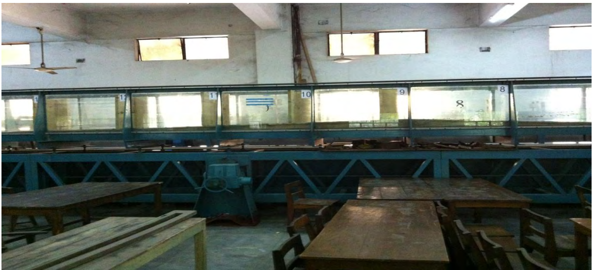
Figure 4.1: Laboratory flume in the hydraulics and river engineering laboratory, DWRE, BUET
