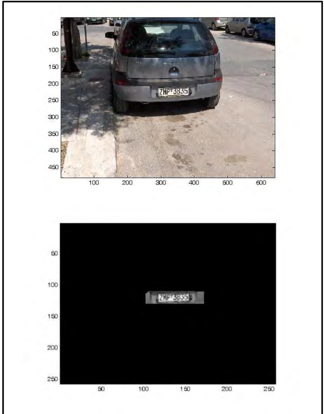
Figure 4.6: a)Original Image and the Detected License Plate
