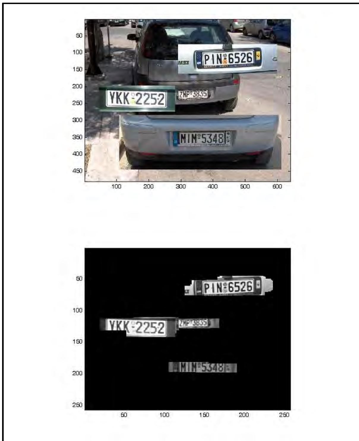
Figure 4.6: b)Image with Multiple License Plates and the Detected Plates
