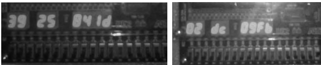
Figure 5.7: Seven segment output of FPGA (1 st 32 bit cipher & 2 nd 32 bit cipher)
