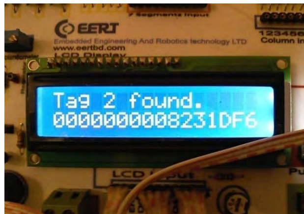
Figure 4.2 Snapshot of displayed RFID Tag number on the LCD screen
