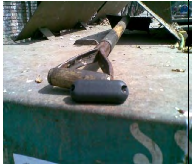
4. RFID Tag is mounted on the container
