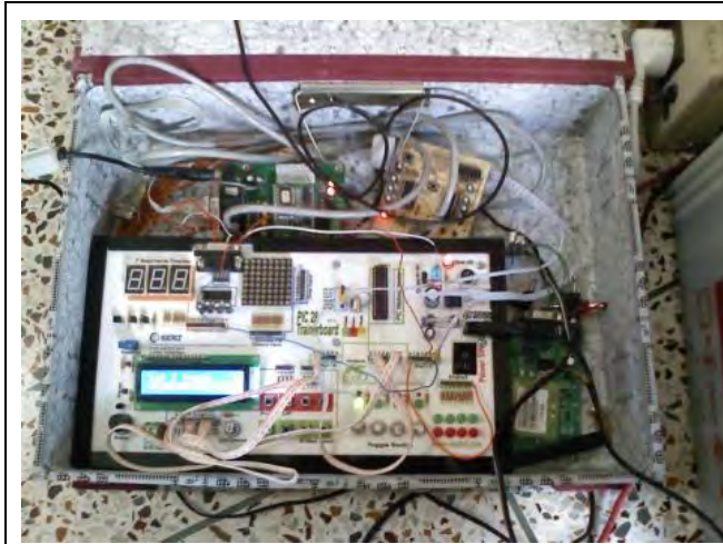
1. Embedded System of solid waste management system
