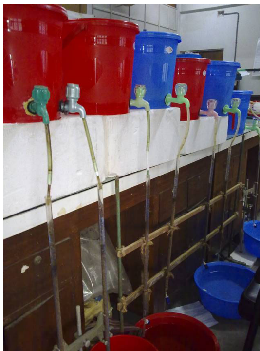
Figure 3.1 Experimental Setup for preparation of filter media with Manganese oxide coatings
