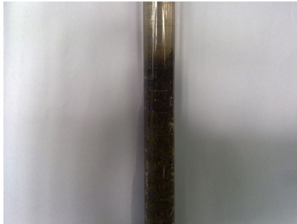
Figure 4.4: Manganese oxide coating formed on sand particles turning them dark (photograph taken after maturation period).
