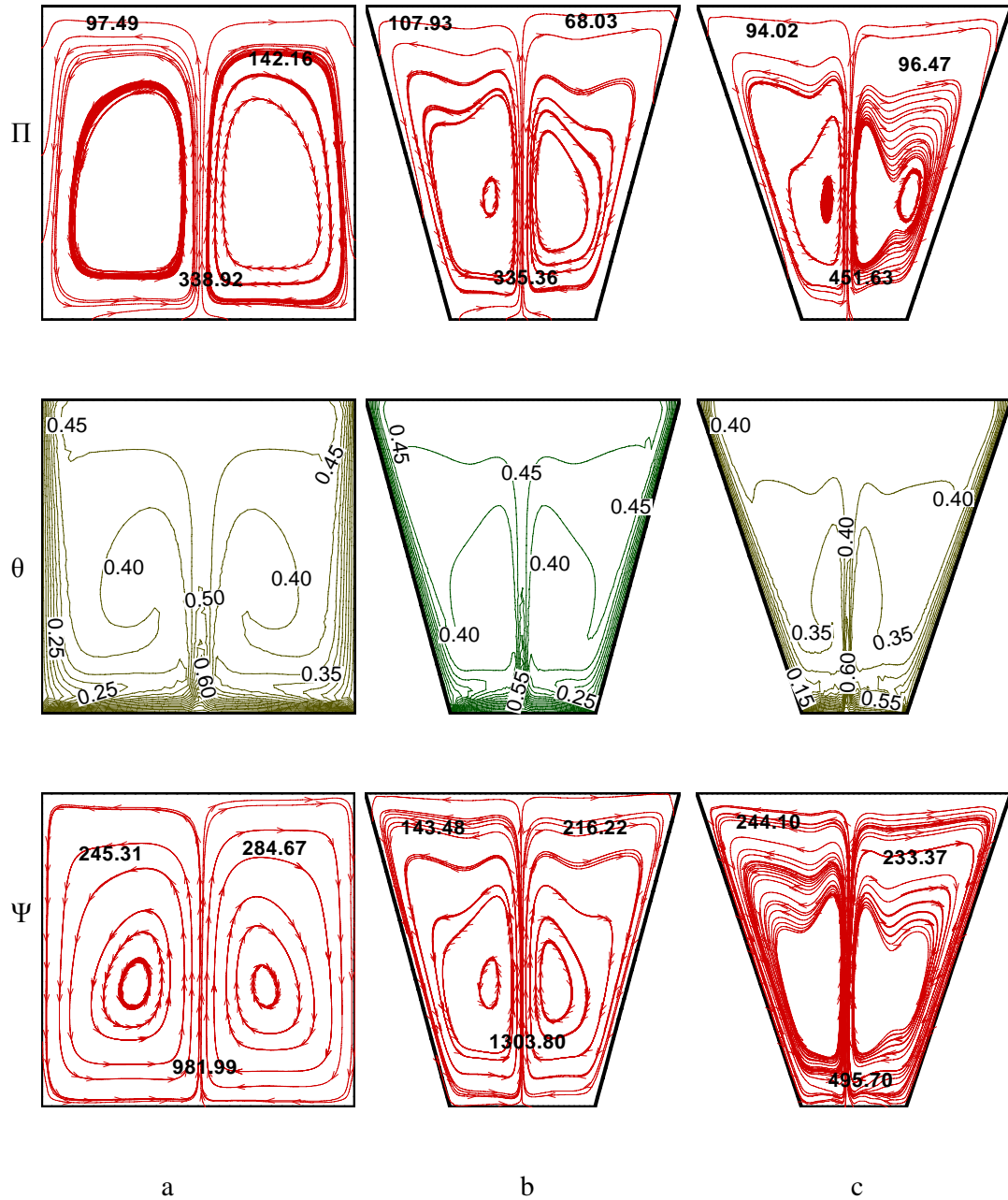
Figure 5.19: Stream function ( \Psi ), temperature ( \theta ), heat function or total heat flux( \Pi ) contours for uniform bottom heating \theta(X,0) = 1 with Pr = 1000 , Ha = 50 and Ra = 10^7 (a) \Phi = 0^\circ (b) \Phi = 30^\circ (c) \Phi = 45^\circ
