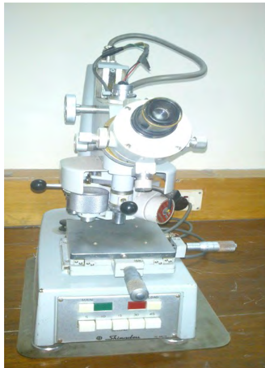
Figure3.7: Hardness testing machine
