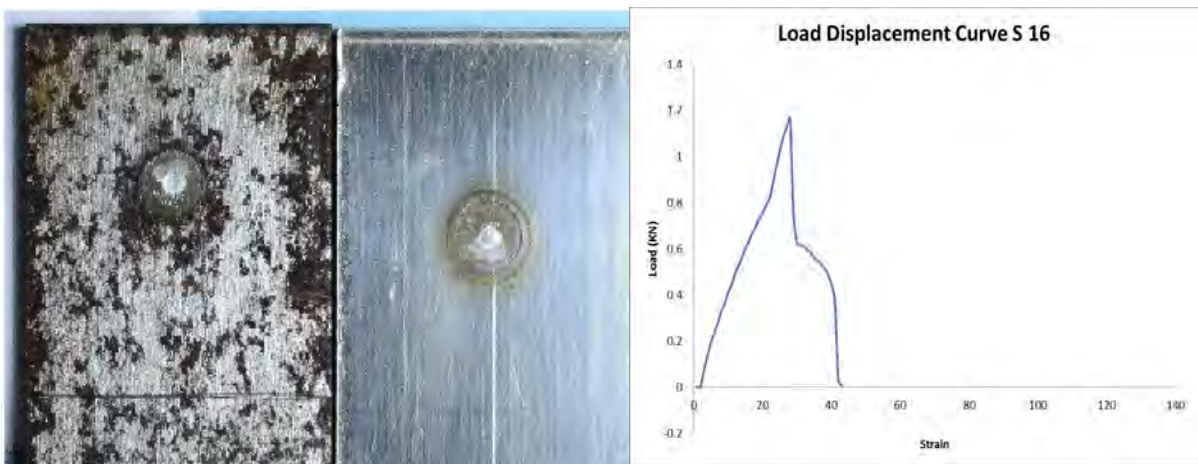
Figure 4.75: Failure mode of sample S-16
