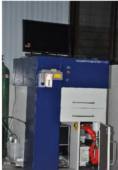
Figure3.1. Optical emission spectrometer
