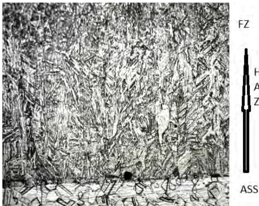
Figure 4.34: coarse columnar grain of weld nugget, 20X.
