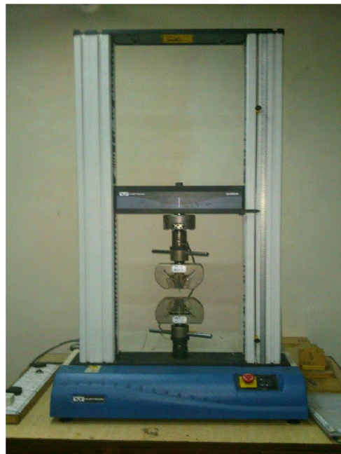
Figure 3.5: Universal testing machine (Instron 3369).
