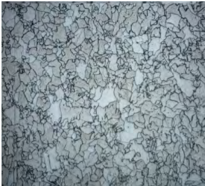
Figure 4.28: Transition Zone in the low carbon steel side, 50X.
