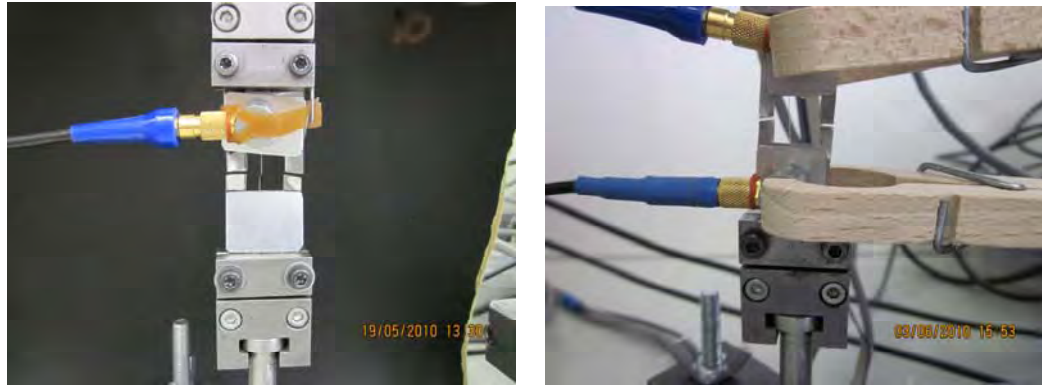
Figure 3-5: Placement of sample holder in the mini tensile machine
