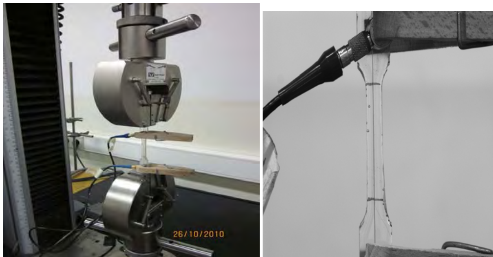
Figure-3-14: Experimental Setup for Dog bone shape sample at Tensile machine with AE Technique
