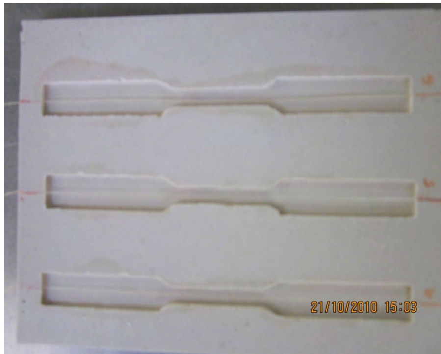
Figure-3-12: Sample with Mold
