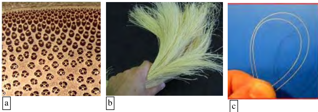
Figure: 3-3: (a) Bamboo culm (b) Bamboo (technical) fibres after mechanical extraction from culm (c) Kink Test of bamboo fibre
