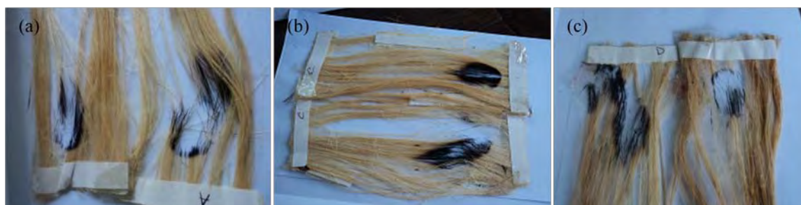
Figure 4.23: Flammability test of (a) 20%FR (b) 25%FR (c) 30%FR treated single jute fiber.
