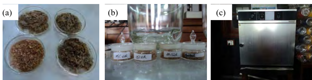
Figure 3.4: Rot retardant (a) chopped jute fiber (b) moisture content measurement and (c) oven.
