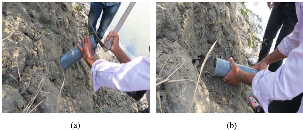
Figure 3.4 Undisturbed soil sample collection procedure (a) insertion of PVC pipe and (b) taking out of PVC pipe with soil sample inside
