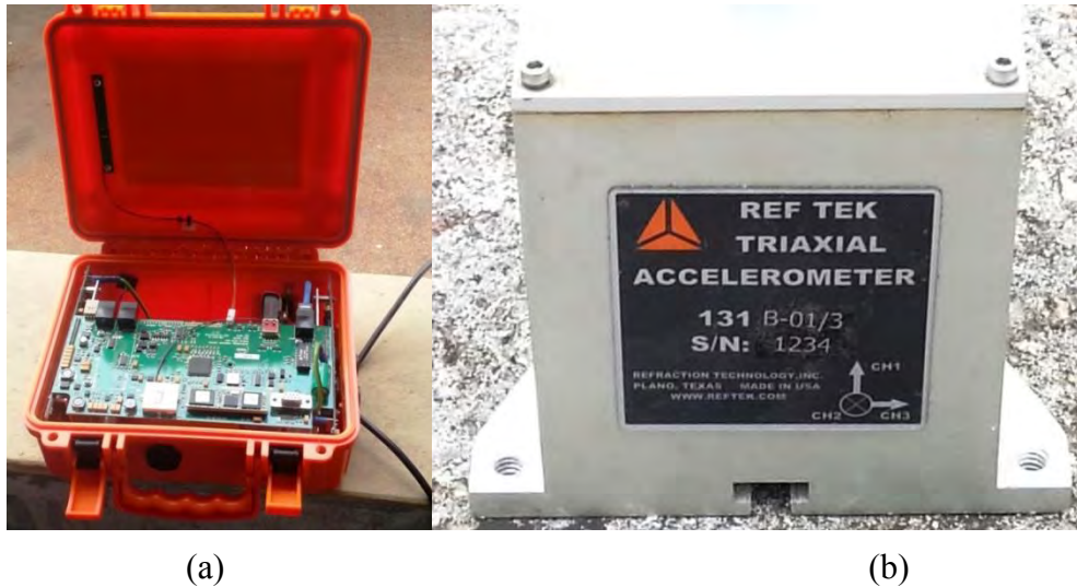
Figure 4.35: (a) The Internal view of the Data Recorder and (b) a Closer View of a Sensor
