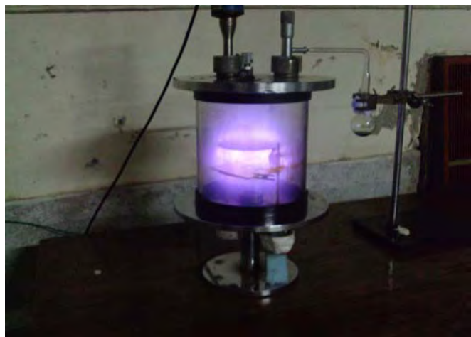
Fig.3.3 Glow discharge plasma during deposition
