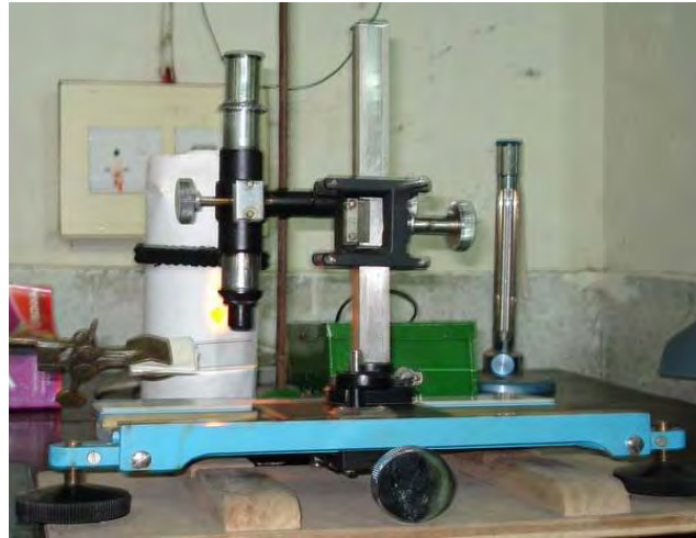
Fig.3.6 Multiple Beam Interferometric set-up in laboratory
