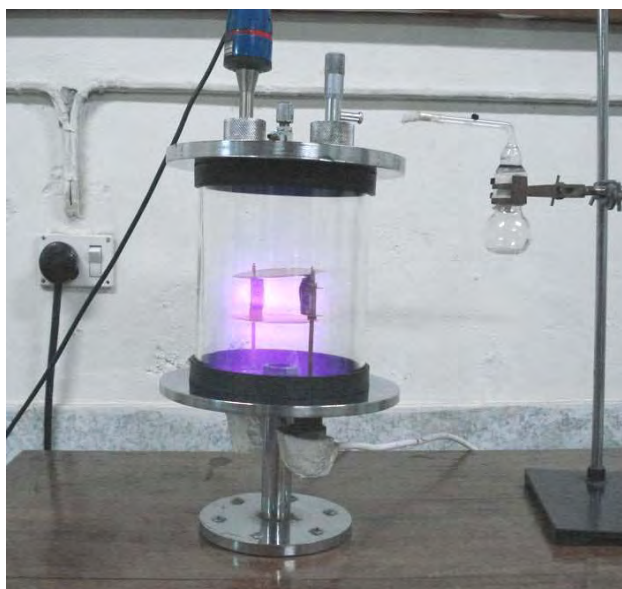
Fig. 3.4 Glow discharge plasma during deposition.
