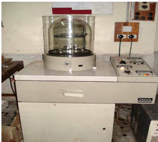
Fig. 3.5 The Edward vacuum coating unit E 306A
