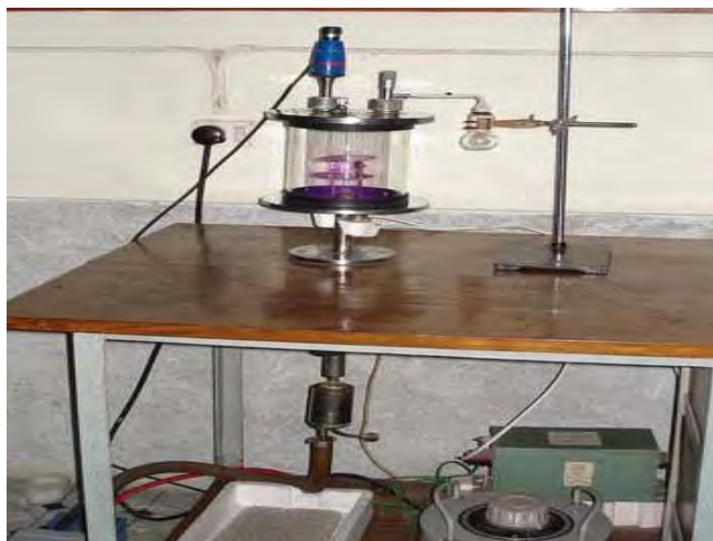
Fig. 3.3 The plasma polymerization set-up
