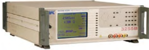
Fig.4.9 Inductance Analyzer (Wayne Kerr) 3255 B
