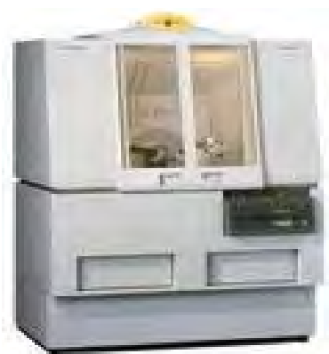
Fig.4.7 X-ray Diffractometer (model: PW 3040-X'Pert PRO Philips) with high temperature attachment.
