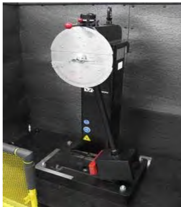
Fig 3.13: Photograph of universal impact testing machine
