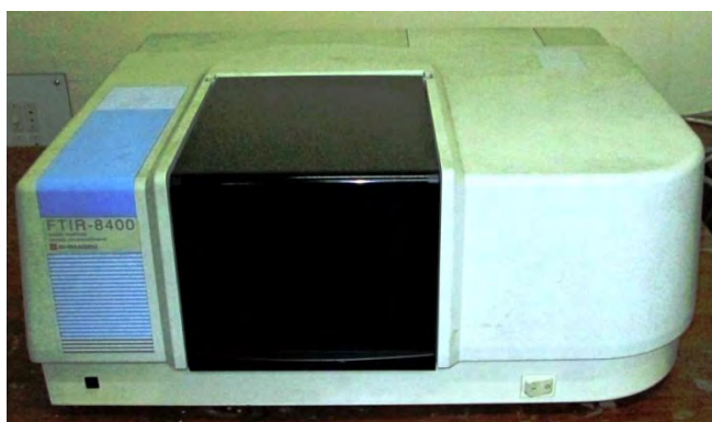
Fig. 3.8: Photograph of FT-IR instrument (Shimadzu FTIR-8400)
