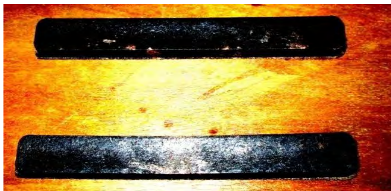
Fig. 3. 7: Photograph of (b) flexural strength test specimen
