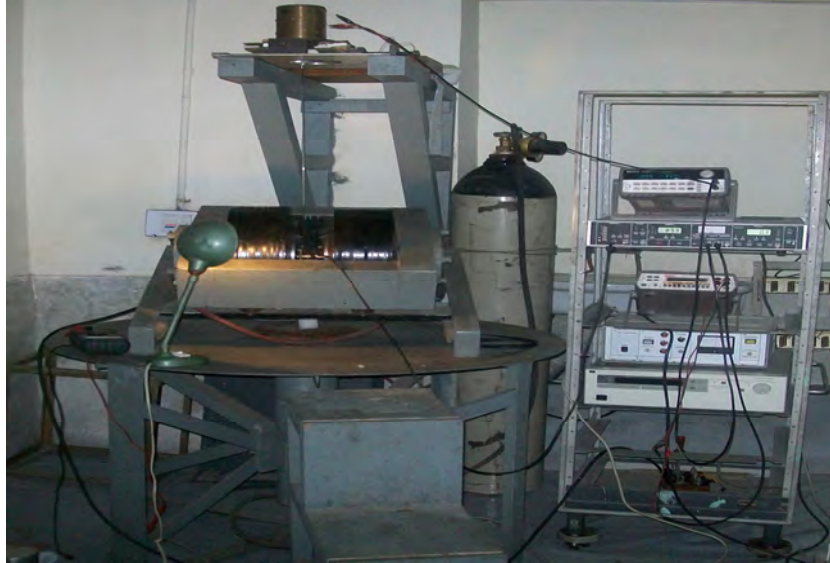
Figure 4.6. Vibrating sample magnetometer (VSM) setup
