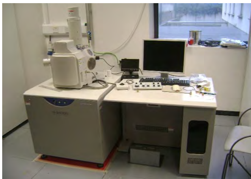
Figure 4.2. External view of Hitachi S-3400N scanning electron microscope
