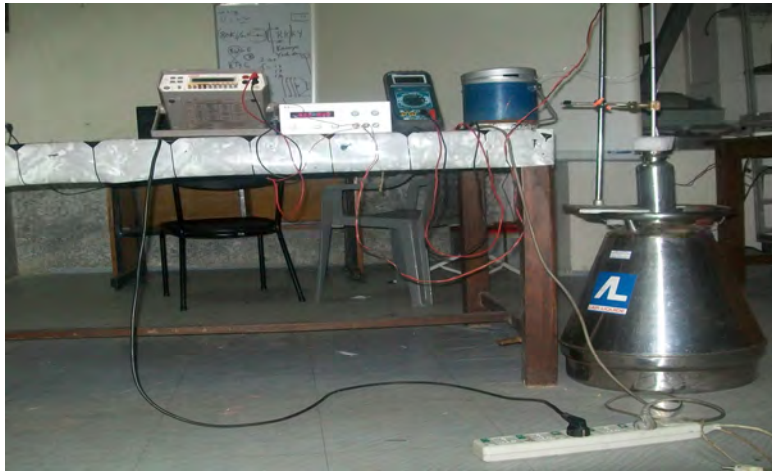
Figure 4.4. Low temperature resistivity measurement setup
